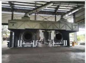
The aluminium rotary furnace operates on the principle of high-temperature rotary melting, providing an effective solution for recycling aluminium. Its primary function is to melt aluminium scrap efficiently, facilitating the separation of impurities and transforming the material into molten aluminium ready for reuse.
