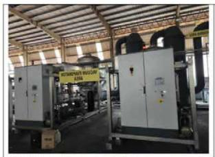
Vacuum evaporation is a process of separating a liquid from a solid or another liquid by using heat under reduced pressure. In this process, the liquid is heated in a vacuum chamber, which reduces the boiling point of the liquid. As a result, the liquid evaporates more easily, leaving behind the solid or another liquid.
